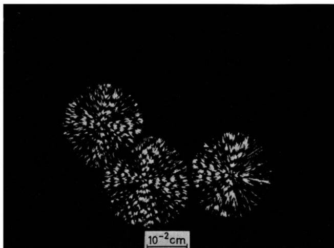
Figure 6 —A spherulitic sample of fraction 5908, produced by an arbitrary heat treatment. Spherulites grown from the melt at 118.4^{\circ}\text{C} for 8 minutes
