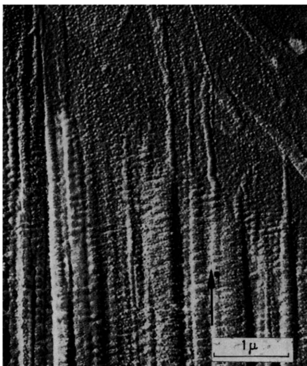
Figure 5 —Blendered microfibrils of Fortisan after etching in a gas discharge six minutes at 3 mA. Arrow indicates fibre axis
