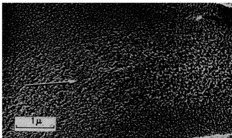
Figure 4 —Etched longitudinal section of a core skin yarn. Arrow indicates fibre axis
