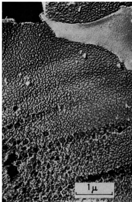
Figure 1 —Portion of an etched transverse section of a core skin yarn. Shadowed with tungsten oxide
